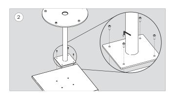
Using the 5/32" hex key, fasten the base sub assembly with  $1/4 - 20 \times 3/4$ " button head cap screw (x4).
