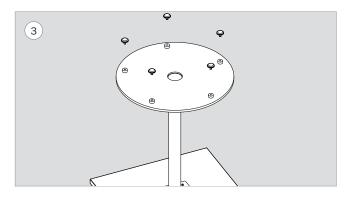
Attach the adjustable glides (x5) to the bottom of the base plate at the lug locations.
